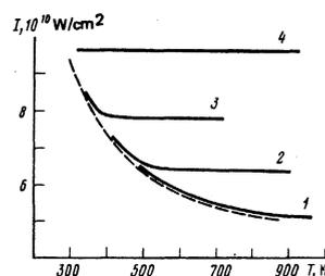
FIG. 2. Temperature dependences of the laser damage threshold at  $\lambda \approx 3 \mu$  and different breakdown probabilities  $P$ : 1)  $P = 0.1$ ; 2)  $P = 0.5$ ; 3)  $P = 0.9$ . Line 4 corresponds to the case when an avalanche is delayed by a shortage of initiating electrons throughout the investigated temperature range. The dashed curve corresponds to the case of a sufficient number of initiating electrons.
