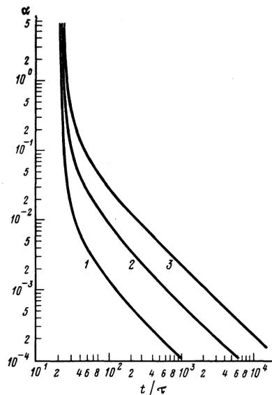
FIG. 1. Solution of Eq. (4) for  $n = 10^{10}$  and three values of the breakdown probability: 1)  $p = 1.0$ ; 2)  $p = 0.5$ ; 3)  $p = 0.9$ .
