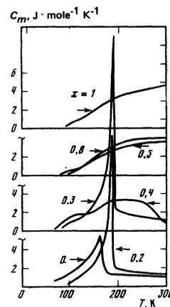
FIG. 2. Magnetic heat capacity of  $\text{Pt}_3\text{Mn}_x\text{Fe}_{1-x}$  alloys as a function of temperature.
