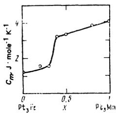
FIG. 4. Magnetic heat capacity of alloys vs. the manganese concentration at  $T = 240$  K.
