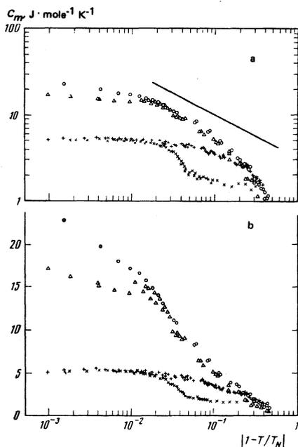
FIG. 3. Magnetic heat capacity of  $\text{Pt}_3\text{Mn}_x\text{Fe}_{1-x}$  alloys as a function of  $|1 - T/T_N|$  in logarithmic (a) and semilogarithmic (b) coordinates. For  $T < T_N$ : +)  $x = 0$ ,  $\Delta$ )  $x = 0.2$ ;  $\circ$ )  $x = 0.3$ . For  $T > T_N$ :  $\times$ )  $x = 0$ . The solid line is a plot of (2) with  $\alpha = 0.5$ .
