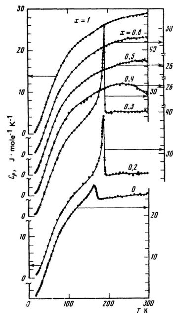
FIG. 1. Heat capacity of  $\text{Pt}_3\text{Mn}_x\text{Fe}_{1-x}$  alloys as a function of temperature.
