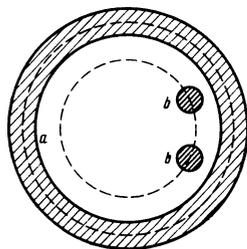
FIG. 4. Schematic representation of the localization of the traveling Langmuir solitons in the plasma-pinch cross section. Dashed circles—resonant magnetic surfaces. The small-amplitude solitons are localized over the entire magnetic surface (a). At high amplitude they are localized around individual force lines (b).
