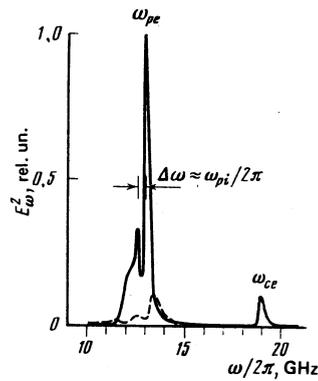
FIG. 3. Intensity spectrum of the microwave fluctuations in a magnetized hydrogen plasma of the "Uragan-2" stellarator in a weak ( $E = 10^{-2} \text{ V/cm}$ —solid line) and in a strong electric field ( $E = 2.5 \times 10^{-2} \text{ V/cm}$ —dashed).
