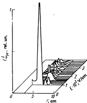
FIG. 2. Redistribution of the intensity  $E_{\omega_{pe}}^2$  of the Langmuir oscillations in a plasma for different values of electric field intensities on the torus loop in the region of the minimum discharge-parameter perturbations introduced by the combined probe. (The dashed line designates the outer-most unperturbed magnetic surface in the "Uragan-2" stellarator; the plasma density distribution is uniform enough within the limits of the separatrix).
