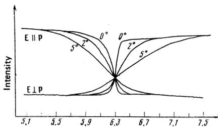
FIG. 3. Variation of light intensity at frequency  $23\,509.5\text{ cm}^{-1}$  with magnetic field (kOe) for various polarizations and angles between  $H$  and  $l$ .
