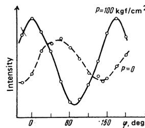
FIG. 2. Effect of uniaxial pressure on polarization of the absorption line.  $\varphi$  is the angle between the electric vector  $E$  of the light and the pressure  $P$ .
