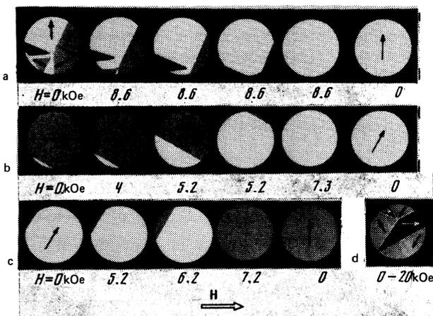
FIG. 1. Change of twin structure of  $RbMnCl_3$  in a magnetic field.
