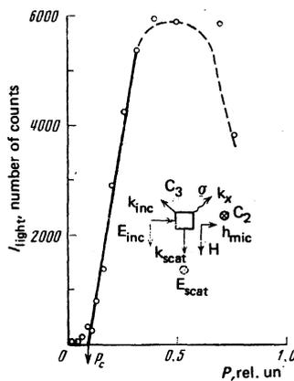
FIG. 4. Variation of the intensity of light scattering by parametric  $x$  magnons with microwave pumping power  $P$  in  $\text{CoCO}_3$  ( $T \lesssim 2\text{K}$ ). Pumping frequency  $\nu_p = 51.02$  GHz.
