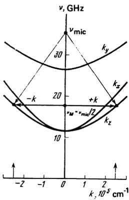
FIG. 5. Sketch illustrating parametric excitation of  $z$  magnons of half frequency in  $\text{CoCO}_3$ , at  $\nu_p \approx 36$  GHz.
