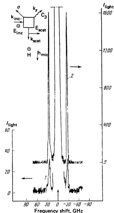
FIG. 2. Spectrum of scattered light ( $\lambda = 632.8$  nm) at  $90^\circ$  in  $\text{CoCO}_3$  ( $T \approx 2$  K) from  $z$  magnons: 1, thermal; 2, parametric, excited by microwave power with  $\nu_p = 51.02$  GHz. The light intensity  $I_{light}$  is given in number of counts. The accumulation time of spectrum 1 is 2000 sec; of spectrum 2, 100 sec.
