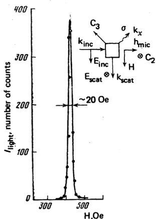
FIG. 3. Variation of the intensity of light scattering by parametric  $x$  magnons with the value of the external magnetic field  $H$  in  $\text{CoCO}_3$  ( $T \lesssim 2\text{K}$ ). Pumping frequency  $\nu_p = 51.02$  GHz.
