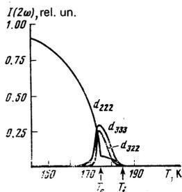
FIG. 1. Temperature dependence of the SHG intensity in the crystal  $(\text{NH}_4)_2\text{BeF}_4$ . The radiation propagates along the  $a$  axis.
