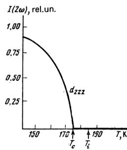
FIG. 2. Temperature dependence of the SHG intensity in the crystal  $(\text{NH}_4)_2\text{BeF}_4$ . The radiation propagates along the  $c$  axis.
