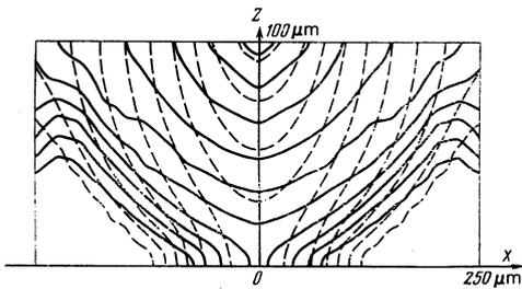
FIG. 2. Isotherms at  $t = 0.3$  nsec ( $q = 3 \cdot 10^{14}$  W/cm<sup>2</sup>,  $b = 50$   $\mu$ m)  $(\nabla \ln n)^{-1} = 25$   $\mu$ m) in a plasma with (solid lines) and without (dashed) allowance for the magnetic-field generation.
