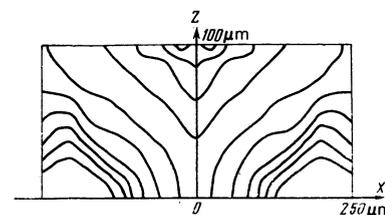
FIG. 5. Isotherms for slow (linear) growth of the heat-release source ( $t = 0.5$  nsec,  $q = 3 \times 10^{14}$  W/cm<sup>2</sup>,  $b = 50$   $\mu$ m, and  $(\nabla \ln n)^{-1} = 25$   $\mu$ m).
