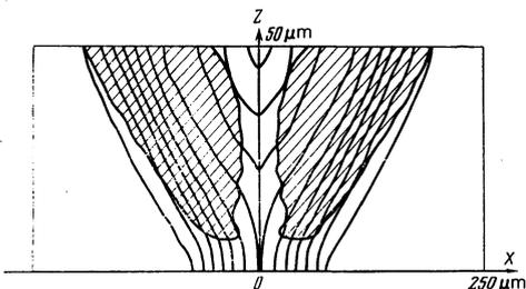
FIG. 3. Isotherms at  $t = 0.45$  nsec ( $q = 10^{14}$  W/cm<sup>2</sup>,  $b = 17$   $\mu$ m,  $(\nabla \ln n)^{-1} = 12.5$   $\mu$ m). The region with  $\omega_e \tau > (\omega_e \tau)^*$  is shaded.
