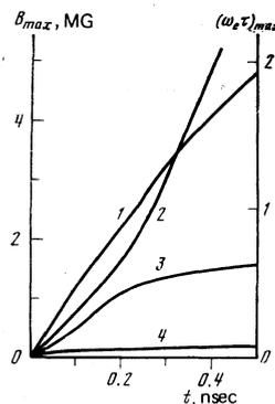
FIG. 1. Maximal values of the magnetic field  $B$  (curves 1, 3) and of the parameter  $\omega_e \tau$  (curves 2, 4) for different dimensions of the heat-release region  $b$ : curves 1, 2— $b = 50 \mu\text{m}$ , 3, 4— $b = 200 \mu\text{m}$ .
