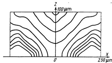
FIG. 4. Isotherms obtained when the heat-release source is turned on instantaneously ( $t = 0.5$  nsec,  $q = 3 \times 10^{14}$  W/cm<sup>2</sup>,  $b = 50$   $\mu$ m,  $(\nabla \ln n)^{-1} = 25$   $\mu$ m).
