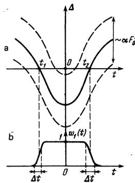
FIG. 1. Time dependence of resonance detuning. The dashed curves correspond to the external values  $\Delta(0)$  at which adiabatic level inversion is possible. b) Probability  $w_1(t)$  of exciting an atom in the adiabatic inversion regime.
