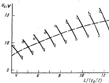
FIG. 7. Values of  $U_c$  for Grandjean bands with large numbers ( $m > 4$ ), calculated from Eq. (12) (solid lines) and experimentally obtained (○) planar orientation,  $p_0=6 \mu$ . The dashed curve corresponds to calculation from the formula of Helfrich-Hurault (2).
