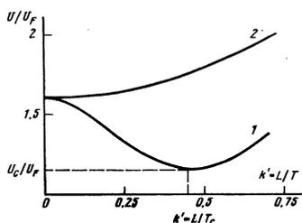
FIG. 3. Lower branch of the solution  $U(k)$  of Eq. (7): the results of a numerical calculation: planar orientation,  $2L/p_0 = 1.25$  (first Grandjean band): curve 1— $\alpha = 0$  (longitudinal domains), curve 2— $\alpha = \pi/2$  (transverse domains).
