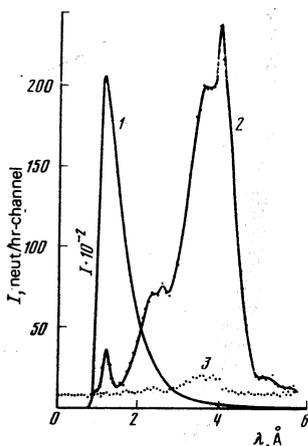
FIG. 3. Spectral dependences of the intensity  $I$  for an isotopic-permalloy filter mirror, layer thickness  $d=100\text{ \AA}$ , glancing angle  $\theta_f=30'$ . 1—spectrum of initial beam incident on the mirror, 2—spectrum of beam reflected in the  $S_-$  state, 3—spectrum of beam reflected in  $S_+$  state.
