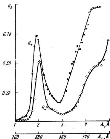
FIG. 2. Dependence of the reflection coefficients  $R_+(\lambda)$  and  $R_-(\lambda)$  for mirror-filter No. 2 based on natural permalloy, with layer thickness  $d = 100 \text{ \AA}$  and glancing angle  $\theta_f = 18'$ .
