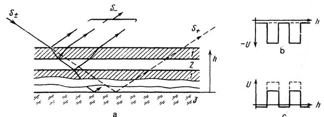
FIG. 1. Periodic filter mirror: a) arrangement of layers: 1—magnetic layers of permalloy 66% Ni + 34% Fe, 2—layers of vanadium, d—glass substrate. The form of the effective potential  $U$  for the spin state  $S_+$  and  $S_-$  when using permalloy made of the isotopes <sup>62</sup>Ni and <sup>54</sup>Fe (b) and permalloy of natural Ni and Fe (c).
