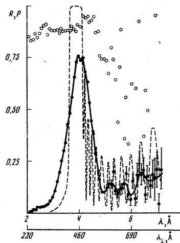
FIG. 4. Dependence of the reflection coefficient  $R(\lambda)$  for filter mirror based on isotopic permalloy with layer thickness  $d=100\text{ \AA}$  and glancing angle  $\theta_f=30'$ . Solid curve—experiment, dashed—theoretical calculation. Points—experimental dependence of the polarization efficiency  $P$  on  $\lambda$ .
