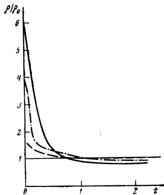
FIG. 6. State-density distribution near  $\frac{1}{4}$  of the band at  $\varphi=0$  and  $\gamma=0.5$  (dashed line),  $\gamma=0.7$  (dash-dot line), and  $\gamma=0.9$  (solid).
