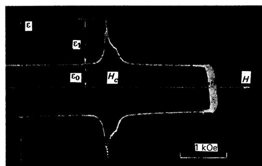
FIG. 2. Dependence of the voltages induced by the change of the external field ( $\mathcal{E}_0$ ) and of the magnetic moment of the crystal ( $\mathcal{E}_1$ ) in a longitudinal induction coil on the magnetic field intensity  $H$ . The upper and lower parts of the curve correspond to the increasing and decreasing sections of the magnetic-field pulse.
