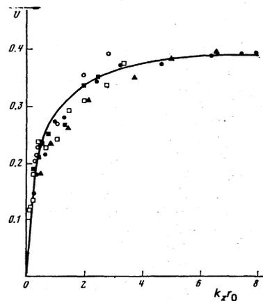
FIG. 4. Experimental dependence of the coefficient of frequency decrease on  $k_z r_0$ :  $\bullet$  -  $P = 3.2 \cdot 10^{-4}$  Torr,  $\circ$  -  $P = 8 \cdot 10^{-5}$  Torr,  $\square$  -  $P = 1.8 \cdot 10^{-4}$  Torr,  $\blacktriangle$  -  $P = 5.4 \cdot 10^{-4}$  Torr,  $\blacksquare$  -  $P = 6.0 \cdot 10^{-5}$  Torr.
