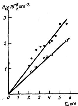
FIG. 2. Dependence of the plasma ion concentration on the system radius.  $\circ$  -  $P = 1.2 \times 10^{-4}$  Torr,  $\bullet$  -  $P = 1.7 \times 10^{-4}$  Torr.
