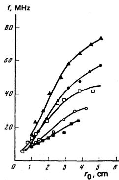
FIG. 3. Dependence of the frequency of the electron oscillations on the system radius:  $\blacksquare$  -  $P = 6 \cdot 10^{-5}$  Torr,  $\circ$  -  $P = 8 \cdot 10^{-5}$  Torr,  $\square$  -  $P = 1.8 \cdot 10^{-4}$  Torr,  $\bullet$  -  $P = 3.2 \cdot 10^{-4}$  Torr,  $\blacktriangle$  -  $P = 5.4 \cdot 10^{-4}$  Torr.
