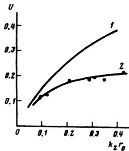
FIG. 5. Dependence of the frequency-decrease coefficient  $U = \omega/\Omega_e$  on the system radius at small  $k_z r_0$ . 1—theory, 2—experiment.
