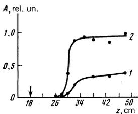
FIG. 6. Dependence of the intensity of the oscillations on the distance to the electron gun at modulation amplitudes equal to zero (curve 1) and 5 V (curve 2). The arrow marks the coordinate of the modulator.  $I=120$  mA,  $U_0=13$  keV,  $p=2 \times 10^{-4}$  Torr,  $f=18$  MHz, diameter 2.5 mm.
