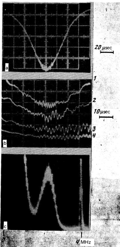
FIG. 1. Oscillograms of signals from a probe moving across the beam (a, b) and spectrum of the current-density oscillations (c). Oscillograms 1, 2, 3, and 4 correspond to different diameters of the beam and are numbered in increasing order of the beam diameter. a) beam current  $I=250$  mA, accelerating voltage  $U_0=18$  kV; b)  $I=30$  mA,  $U_0=6.5$  kV; c)  $I=180$  mA,  $U_0=20$  kV,  $p=5 \times 10^{-4}$  Torr.
