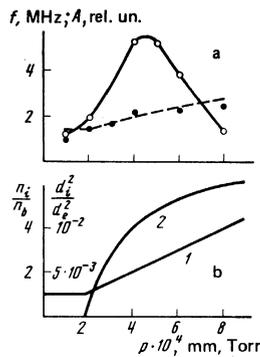
FIG. 7. Effect of air pressure on the parameters of a beam plasma at  $U_0=13$  keV, diameter 2.5–3 mm (b) and on the experimental values of the frequency (●) and of the amplitude (○) of the oscillations at  $U_0=14$  keV,  $I=120$  mA, diameter 3 mm (a). Curve 1— $d_i^2/d_e^2$ , 2— $n_i/n_b$ .
