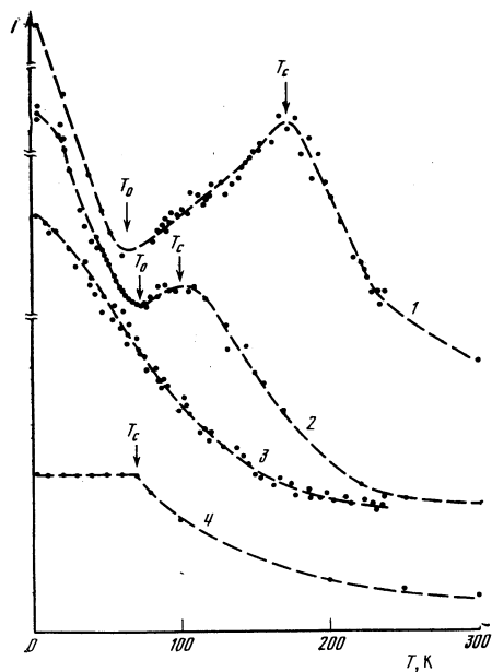
FIG. 1. Temperature variation of the intensity I of neutron scattering at angle 2\theta = 45' . 1, 7.5% V; 2, 10.3% Cr; 3, 10.9% Cr; 4, 9.8% Mn.
