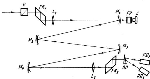
FIG. 1. Measurement setup:  $P$ —polarizer,  $FR_1$  and  $FR_2$ —Fresnel rhombs,  $L_1$  and  $L_2$ —lenses,  $M_1$ – $M_4$ —spherical mirrors,  $FR$ —Fabry-Perot interferometer,  $C$ —photographic camera,  $BP$ —birefringent prism;  $PD_2$  and  $PD_3$ —calorimeters.
