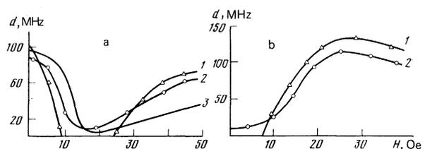
FIG. 3. a) Plots of  $d(H)$  for resonator configuration I and  $p=1.5$  Torr, curve 1—for  $\omega_{12}=40$  MHz, 2—for  $\omega_{12}=80$  MHz, 3—for  $\omega_{12}=45$  MHz (calculated dependence), b)  $d(H)$  for configuration II of the resonator and  $p=1.5$  Torr, curve 1—for  $\omega_{12}=35$  MHz, 2—for  $\omega_{12}=60$  MHz.
