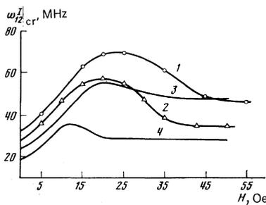
FIG. 1. a) Dependence of  $\omega_{12cr}^I$  on  $H$ : curves 1, 2—experimental (1— $p=1.5$  Torr, 2— $p=1$  Torr); curves 3, 4—calculation (3— $p=2$  Torr, 4— $p=1$  Torr).
