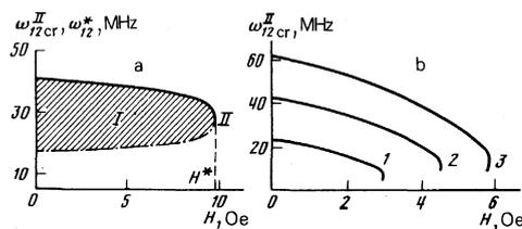
FIG. 2. Experimental plots of  $\omega_{12cr}^{II}$  (solid line) and  $\omega_{12}^*$  (dash-dot) against  $H$  at  $p=1.8$  Torr. I—single-mode generation region, II—stable two-mode generation region. b) Calculated plots of  $\omega_{12cr}^{II}$  against  $H$ . Curve 1— $p=1.0$  Torr, 2— $p=1.5$  Torr, 3— $p=2.0$  Torr.
