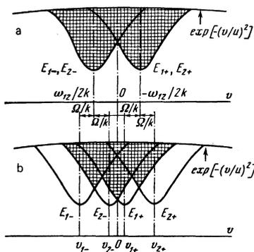
FIG. 5. Illustration of the behavior of  $\omega_{12}^{II cr}(H)$ , the cross hatching shows the overlap of the "holes" in a zero (a) and a nonzero (b) magnetic field.
