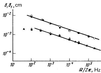
FIG. 6. Dependences of the depth of the skin layer  $\delta$  (O, ●) and of the thickness of the superconducting layer  $\delta_1$  (Δ, ▲) on the frequency of the alternating field: O - In-1, ● - In-4; Δ - In-1, ▲ - In-4,  $H_~ = 30$  Oe,  $H_c = 75$  Oe,  $H_0 = 75$  Oe, ▲ - In-4,  $H_~ = 67$  Oe,  $H_c = 75$  Oe,  $H_0 = 75$  Oe. The lines are proportional to  $\omega^{-1/2}$ .
