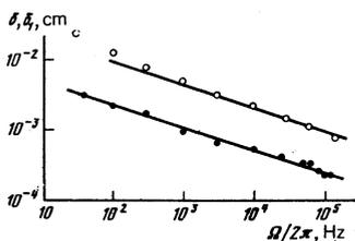
FIG. 5. Depth of skin layer  $\delta$  (O) and thickness of superconducting layer  $\delta_1$  (●) vs the frequency of the alternating field for Sn-3. The points for  $\delta_1$  were obtained at  $H_0 = 225$  Oe,  $H_c = 230$  Oe,  $H_~ = 37$  Oe. The lines are proportional to  $\omega^{-1/2}$ .
