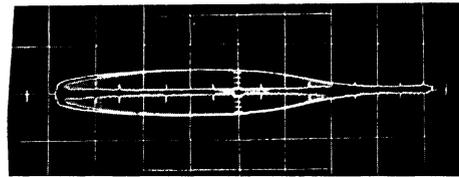
FIG. 2. Typical photograph from oscilloscope screen. The ordinates represent the bridge-unbalance voltage, and the abscissas the alternating component of the magnetic field parallel to the surface of the plate ( $H = H_0 + H_m \sin \Omega t$ ,  $H_0 = 23$  Oe,  $H_m = 6.3$  Oe,  $H_c = 30$  Oe,  $H_c = 28.5$  Oe,  $\Omega/2\pi = 96 \times 10^3$  Hz,  $\omega/2\pi = 10.2$  MHz). The experimental conditions correspond to plateau  $b$  on curve 2 of Fig. 10 below.
