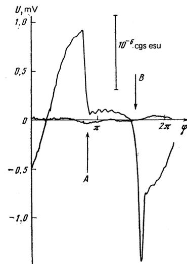
FIG. 3. Voltage on receiving coil as a function of the phase of the alternating field. Sample Sn-3,  $f = \Omega/2\pi = 146 \times 10^3$  Hz,  $H_0 = 40$  Oe,  $H_c = 54$  Oe,  $H_m = 40$  Oe. For comparison, a plot is shown obtained under conditions when the entire sample is superconducting. The appearance of a small voltage in this case is due to insufficient cancellation of the signal from the gap between the sample and the receiving coil.
