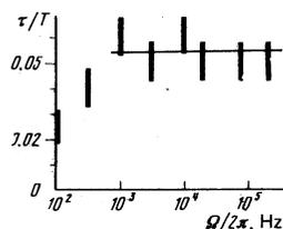
FIG. 7. Plot of  $\tau/T$  against the frequency of the alternating field for In-4,  $H_c = 75$  Oe,  $H_0 = 75$  Oe,  $H_~ = 67$  Oe.
