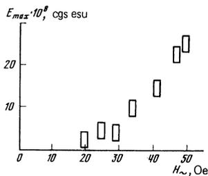
FIG. 4. Dependence of the maximum value of the electric field in the layer on the amplitude of the alternating field for Sn-3,  $H_0 = 40$  Oe,  $H_c = 54$  Oe,  $\Omega / 2\pi = 146$  kHz.
