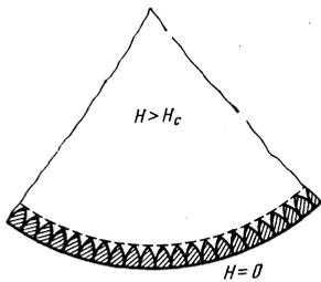
FIG. 1. Cut through a cylindrical sample by a plane perpendicular to the cylinder axis. The superconducting regions are shaded.
