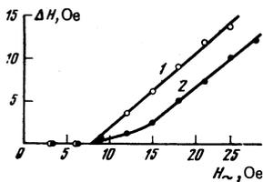
FIG. 8. Dependence of the shift of the superconducting transition on the amplitude of the alternating field in a parallel dc field and in a field inclined to the sample axis. Sample Sn-1,  $H_c = 45.5$  Oe,  $\Omega/2\pi = 1$  kHz. Curve 1 corresponds to an inclination angle  $\psi = 0$ , and curve 2 to  $\psi = 25^\circ$ .
