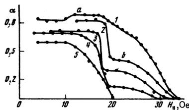
FIG. 10. Dependence of  $\alpha$  on  $H_{\parallel}$  at different  $H_{\perp}$  for sample In-4,  $H_c = 28.5$  Oe,  $H_{\perp} = 21$  Oe,  $f = 96$  kHz,  $\omega/2\pi = 10.2$  MHz. Curves: 1)  $H_{\perp} = 5.1$ ; 2) 6.3; 3) 6.6; 4) 7.8; 5) 9.8 Oe.
