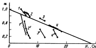
FIG. 11. Dependence of  $\alpha$  on  $H_{\perp}$  on plateau *a* (curves 1-4) and plateau *b* (curves 1'-4'). Sample In-4,  $H_c = 28.5$  Oe,  $\omega/2\pi = 10.2$  MHz. Curves 1 and 1' correspond to  $f = 114$  kHz,  $H_{\perp} = 30$  Oe; 2, 2' - for  $f = 96$  kHz and  $H_{\perp} = 21$  Oe; 3, 3' - for  $f = 11.6$  kHz,  $H_{\perp} = 30$  Oe; 4, 4' - for  $f = 116$  Hz,  $H_{\perp} = 30$  Oe.
