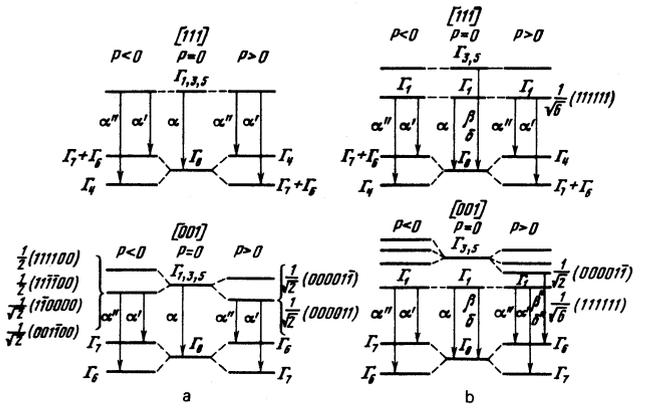
FIG. 4. Splitting of states of MIPC bound on a simple acceptor (a) and donor (b) in silicon under uniaxial tension ( $P < 0$ ) and compression ( $P > 0$ ) along the axes [111] and [001].
