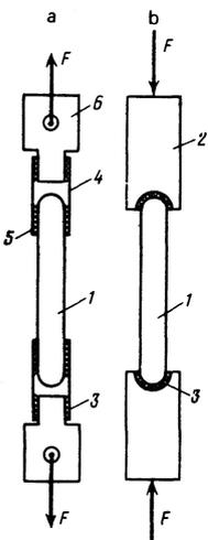
FIG. 1. Diagram of installation for uniaxial tension (a) and compression (b) of silicon samples: 1—sample, 2—plunger, 3—50% Sn + 50% Pb solder, 4—copper-foil vessels, 5—epoxy resin, 6—lugs.
