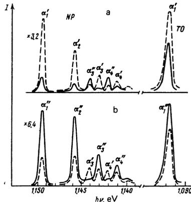
FIG. 5. Spectral distribution of NP and TO components of the emission of MEIC bound on atoms of phosphorus in silicon at 2 K, polarized parallel (solid line) and perpendicular (dashed) to the direction of deformation along the [111] axis: a—tension,  $P = -275 \text{ kg/cm}^2$ , b—compression,  $P = 275 \text{ kg/cm}^2$ .
