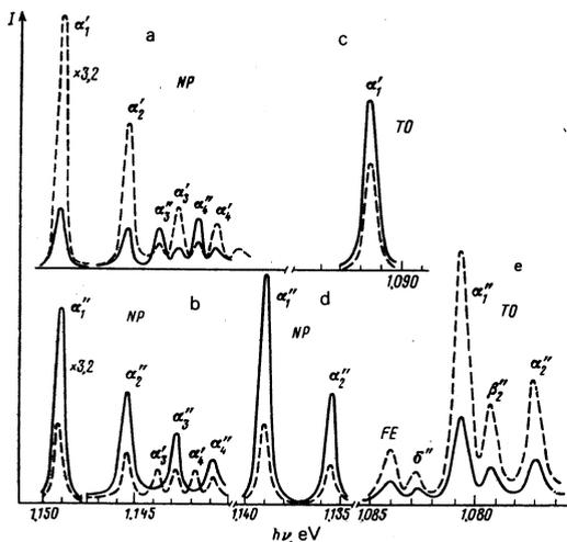
FIG. 6. Spectral distribution of the emission of MEIC bound on phosphorus atoms in silicon at 2 K, polarized parallel (solid line) and perpendicular (dashed) to the direction of deformation along the [001] axis: tension,  $P = -250 \text{ kg/cm}^2$ , a) NP component, c) TO component; compression: b)  $P = 250 \text{ kg/cm}^2$ , NP component,  $P = 2000 \text{ kg/cm}^2$ , d) NP component, e) TO component.
