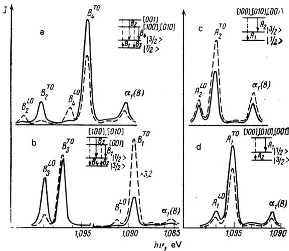
FIG. 2. Splitting of exciton levels in silicon and spectral distribution of TO and LO components of the emission of free excitons at 2 K, polarized parallel (solid line) and perpendicular (dashed) to the deformation; along the [001] axis: a—tension,  $P = -690 \text{ kg/cm}^2$ , b—compression,  $P = 1000 \text{ kg/cm}^2$ ; along the [111] axis: c—tension,  $P = -280 \text{ kg/cm}^2$ , d—compression,  $P = 630 \text{ kg/cm}^2$ .
