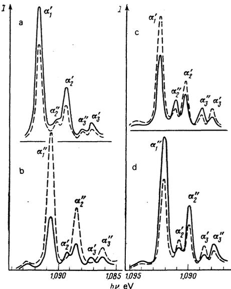
FIG. 8. Spectral distribution of TO component of the emission of MEIC bound on boron atoms in silicon at 2 K, polarized parallel (solid line) and perpendicular (dashed) to the direction of deformation along the [001] axis: a—tension,  $P = -220$  kg/cm<sup>2</sup>, b—compression,  $P = 220$  kg/cm<sup>2</sup>; along the [111] axis: c—tension,  $P = -260$  kg/cm<sup>2</sup>; d—compression,  $P = 260$  kg/cm<sup>2</sup>.
