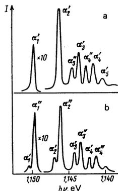
FIG. 7. NP component of the emission spectrum of MEIC bound on phosphorus atoms in silicon under uniaxial deformation along the [111] axis: a—tension,  $P = -275 \text{ kg/cm}^2$ , 2 K; b—compression,  $P = 275 \text{ kg/cm}^2$ , 4.2 K.
