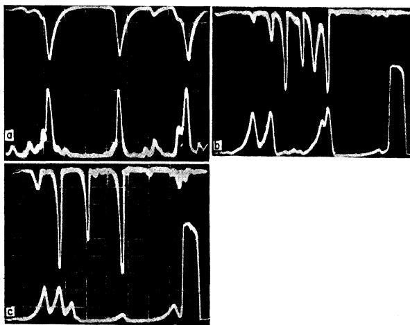
FIG. 8. Oscillograms of the rf pulses from the same probe at two frequencies close to the electron Langmuir frequency: f_1 = 500 MHz and f_2 = f_1 + \Delta f for three values of the frequency shift \Delta f : a—5 MHz, b—15 MHz, c—25 MHz. The time base is 5 \mu\text{s}/\text{division} . The pulse at the end of the oscillograms is connected with the switching-off of the beam.
