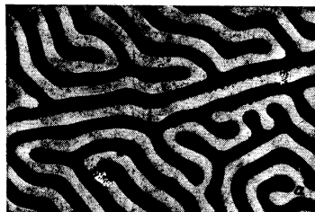
FIG. 1. Pinning by dislocations (light circles) of walls of stripe domains of a film in the demagnetized state.
