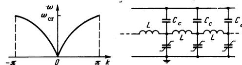
FIG. 1. Diagram of investigated LC network and its dispersion characteristic.
