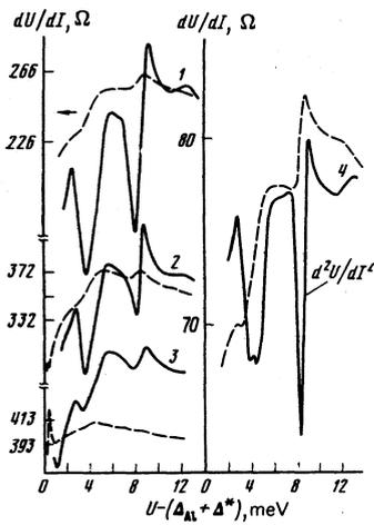
FIG. 3. Manifestation of phonon singularities of lead in the tunnel conductance of the same Al-I-CuCl/Pb structures as in Fig. 2, but at  $T=1.1$  °K. Here and later, the dashed curves represent the  $dU/dI-U$  dependences and the continuous curves are the  $d^2U/dI^2-U$  dependences. Here and in the remaining figures, the energies are measured from the sum of the gaps  $\Delta_{Al} + \Delta_{N/Pb} = \Delta_{Al} + \Delta$ .
