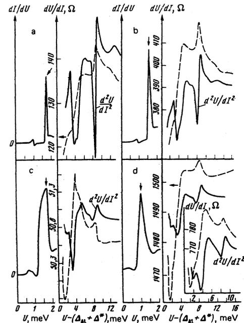
FIG. 5. Changes in the tunnel characteristics of Al-I-Cu/Pb systems with  $d_{Cu}$  (Å): a) 15; b) 50; c) 100; d) 200.  $T=1.1$  °K. The inset shows the characteristics of an Al-I-Ag/Pb structure with  $d_{Ag} = 150$  Å.
