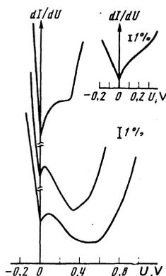
FIG. 1. Anomalous behavior of the tunnel conductance of three Al–I–CuCl/Pb structures subjected to high voltages across the barrier at  $T=77^\circ\text{K}$ . The inset shows the same dependence for an Al–I–Pb structure (here and later, the curves are copies of the experimental records).
