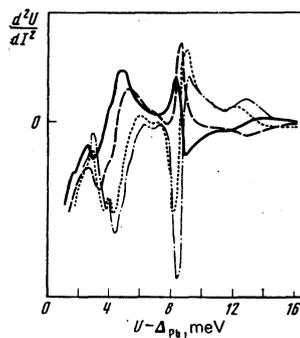
FIG. 6. Manifestation of the phonon structure of lead in the  $d^2U/dI^2-U$  dependences of the second derivatives. The calculations are carried out in the model of Ref. 2 for  $v_N = 1 \times 10^8$  cm/sec and  $d_N$ : the chain curve corresponds to 30 Å, the dotted curve to 100 Å, the dashed curve to 300 Å, and the continuous curve to 500 Å. Similar behavior is predicted by the model of Ref. 20 with  $\Gamma = 25, 15, 5,$  and 2 meV.
