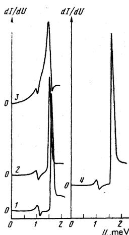
FIG. 2. Tunnel conductance of Al–I–CuCl/Pb structures in the energy range of the superconducting gaps of aluminum and lead with films of copper chloride of the following thickness  $d_{\text{CuCl}}$  (Å): 1) 16; 2) 65; 3) 180; 4) Al–I–Pb structure.  $T=1.1^\circ\text{K}$ .
