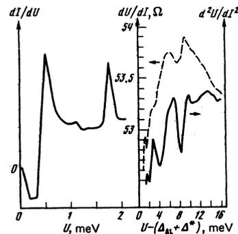
FIG. 4. Tunnel characteristics of Al-I-Bi<sub>33</sub>Sb<sub>67</sub>/Pb structures with  $d_{BiSb} = 1000$  Å at  $T=1.1$  °K.
