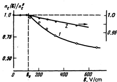
FIG. 2. Dependence of the populations of levels of depth 0.24 eV (curve 1) and 0.4 eV (curve 2) on the field amplitude. Frequency 100 kHz. The continuous curves are the theoretical dependences,
