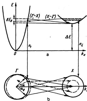
FIG. 3. Intervalley electron transition scheme. The dependences  $E(k)$  are given at the top (Fig. 3a) and the constant-energy surfaces near the  $\Gamma$  and  $X$  points of the Brillouin zone are given at the bottom (Fig. 3b).
