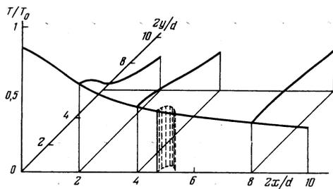
FIG. 1. Temperature distribution in a planar supersonic stream. The  $x$  axis coincides with the direction of motion of the gas. The  $y$  axis is perpendicular to the plane of symmetry of the stream and the origin is located at the edge of a supersonic nozzle;  $d$  is the height of the nozzle throat.
