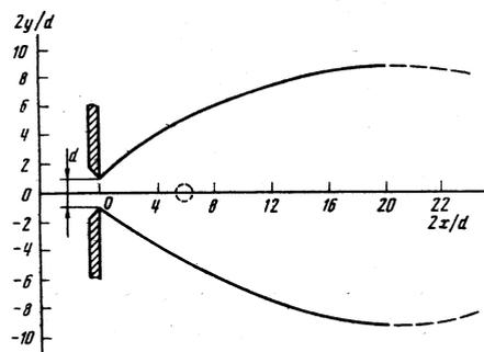
FIG. 2. Schematic representation of the observation conditions. The boundaries of a planar jet are shown up to the region with maximum broadening. The dashed circle identifies the position of the microwave beam.
