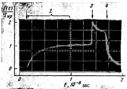
FIG 2. Oscillogram of experiments: 1—emergence of shock wave into the gas, 2—section where the radiation grows to saturation, 3—collision of shock wave front with transparent partition, 4—start of destruction of partition by the target material.
