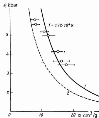
FIG. 4. Comparison of the bounded-atom model with the thermodynamic measurements:  $\circ$ —results of Ref. 13 referred to the isotherm  $T = 1.72 \times 10^4 \text{ K}$ ; 1—calculation by the bounded-atom model, 2—calculation by the Debye-Huckel model.<sup>30</sup>
