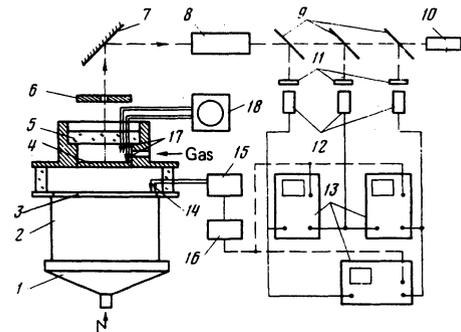
FIG 1. Experimental setup: 1—detonation lens, 2—explosive charge, 3—striker, 4—target, 5—transparent partition, 6—diaphragm, 7—mirror, 8—optical system, 9—semitransparent mirrors, 10—adjusting laser, 11—interference light filters, 12—photomultipliers, 13—recording oscillographs, 14—electric contacts that start the oscillographs, 15—pulse-shaping circuit, 16—delay line, 17—electric contacts for the measurement of the shock wave velocity, 18—OK-15 oscilloscope.
