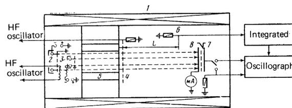
FIG. 3. Schematic illustration of the experimental system: 1—solenoid; 2, 3—electron guns; 4—feeding electrode; 5—bunching channel; 6—mobile probe; 7—collector of the electrostatic analyzer; 8—collector.
