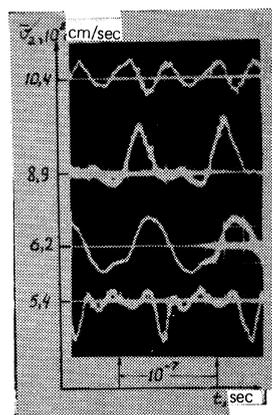
FIG. 4. Oscillations in the circuit of the mobile probe as functions of the mean velocity of the additional  $\bar{v}_2$ ;  $v_1 = 1.04 \times 10^9$  cm/sec,  $f = 11.8$  MHz,  $L = 60$  cm.
