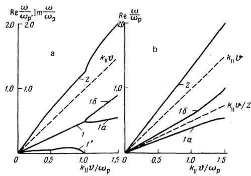
FIG. 1. Dispersion curves for the beam-plasma system when the densities are equal: (a) curve 1— $\operatorname{Re}(\omega/\omega_p)$ , 1'— $\operatorname{Im}(\omega/\omega_p)$ , 2—constant intensity wave;  $\sigma^2 = k_{\perp} v_1 / \omega_p)^2 = 7.0$ . (b) Curves 1a and 1b— $\operatorname{Re}(\omega/\omega_p)$ , 2—constant intensity wave;  $\sigma^2 = 8.0$ ,  $\operatorname{Im}(\omega/\omega_p) = 0$ .
