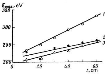
FIG. 8. Maximum energy of trapped particles as a function of distance  $L$ : 1—left-hand current peak; 2—right-hand current peak, both for  $\bar{v}_2 = 5.4 \times 10^8$  cm/sec; 3— $\bar{v}_2 = 8.9 \times 10^8$  cm/sec.
