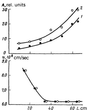
FIG. 6. Amplitude  $A$  and velocity  $v$  of BGK waves as functions of distance  $L$ : (1)  $\bar{v}_2 = 5.4 \times 10^8$  cm/sec, (2)  $\bar{v}_2 = 8.9 \times 10^8$  cm/sec.
