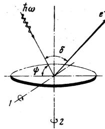
FIG. 1. Position of sample in HP 5950A spectrometer.
