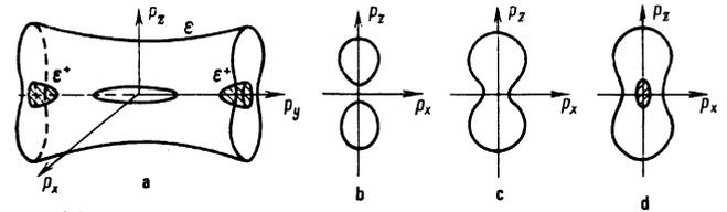
FIG. 6. Fermi surface at  $|\eta| < q^2/8m_{||} - J$  (a) and its sections at  $p_y = 0$  (b),  $[2m_2(q^2/8m_{||} - |\eta| - J)]^{1/2} < p_y < [2m_2(q^2/8m_{||} - |\eta| + J)]^{1/2}$  (c) and  $p_y > [2m_2(q^2/8m_{||} - |\eta| + J)]^{1/2}$  (d).
