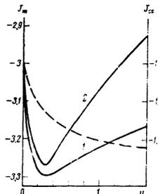
FIG. 1. Variation of the characteristic functions  $J_m$  and  $J_\alpha$  with the normalized square of the wave number,  $u = (k/k_0)^2$ . 1, first approximation to  $J_m(u)$ ; 2, second approximation to  $J_m(u)$ ; dotted curve,  $J_\alpha(u)$ .
