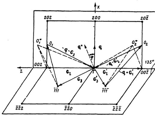
FIG. 1. Splitting of a three-particle singularity when the phonon wave vector  $\mathbf{q}$  is inclined at an angle  $\varphi$  relative to the  $[100]$  direction.
