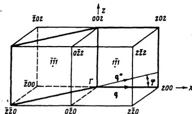
FIG. 2. Reciprocal lattice cell of Al. The thick lines identify the planes in Fig. 1.
