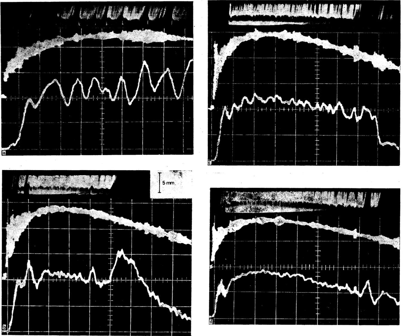
FIG. 1. Recoil force (lowest traces, plotted on a scale of 0.05 V/div. in cases a-c and 0.1 V/div. in case d), laser pulse envelope (upper trace) and plasma radiation (streak patterns at top of figure) obtained for different values of the incident radiation power  $N_{\max}$  (kW): a) 36; b) 40; c) 43; d) 53. Horizontal scales: 50  $\mu\text{sec}/\text{div}$ . (a) and 100  $\mu\text{sec}/\text{div}$ . (b-d). The spatial scale of the streak patterns is shown Fig. 1b.
