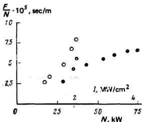
FIG. 4. Dependence of the ratio  $F/N$  on the incident radiation power in the presence ( $\bullet$ ) and absence ( $\circ$ ) of a plasma.
