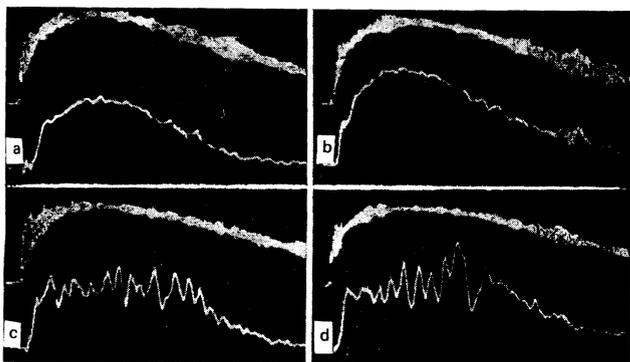
FIG. 3. Recoil force (0.02 V/div. in case a, 0.1 V/div. in case b, and 0.05 V/div. in cases c and d) recorded for different incident radiation intensities  $I$  ( $\text{MW}/\text{cm}^2$ ): a) 1.1; b) 4.1; c), d) 2. Horizontal scale: 100  $\mu\text{sec}/\text{div}$ .
