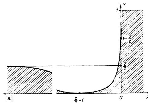
FIG. 2. Region of existence of ferromagnetism (shaded) on amorphization of an ideal magnet with an anisotropic distribution of exchange bonds.
