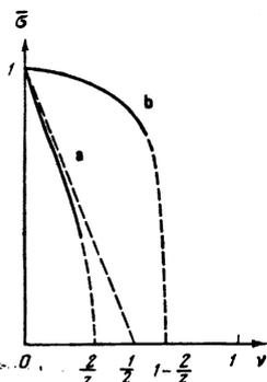
FIG. 1. Variation of the relative magnetization  $\bar{\sigma}$  with the concentration  $\nu$  of antiferromagnetic  $K$  bonds: a, when  $|\lambda| = |K|/J = \infty$ ; b, when  $|\lambda| = 0$ .
