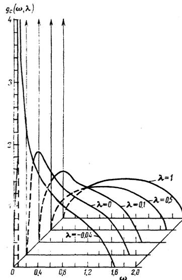
FIG. 4. Density of spin-wave states  $g_c(\omega)$  of an amorphous isotropic ferromagnet, in the CPA, for several values of  $\lambda$  ( $\nu = 1/3$ ).
