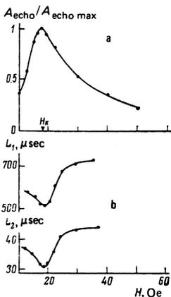
FIG. 4. Spin-echo amplitude as a function of field  $H$  (a) and graphs of  $L_1(H)$  and  $L_2(H)$  (b).
