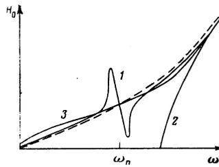
FIG. 1. FMR (AFMR) resonance field  $H_0$  as a function of frequency  $\omega$  in the case of interaction with NMR (curve 1) and in the absence of this interaction (broken curve). The eigenfrequencies are plotted for  $\Gamma_e \ll \omega_q \ll \omega_n$  (curve 2) and  $\omega_q \ll \Gamma_e \ll \omega_n$  (curve 3).
