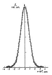
FIG. 2. Distribution of the intensity in a transverse cross section through a laser beam at the entry to a nonlinear medium: the points are the experimental results and the continuous curve is a Gaussian distribution.
