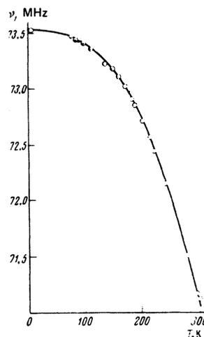
FIG. 3. Temperature dependence of the NMR frequency for hematite.
