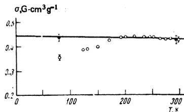
FIG. 2. Temperature dependence of the specific weakly ferromagnetic moment: O—after slow cooling from 1300°C, ●—after quenching at 1300°C. Solid curve—temperature dependence of sublattice magnetization (the curve is “normalized” to the value of  $\sigma$  at room temperature).
