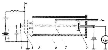
FIG. 1. Schematic diagram of experimental setup: 1—cathode; 2—grid; 3—anode; 4—microwave signal; 5—electron collector; 6—plasma chamber; 7—probe.
