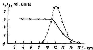
FIG. 9. Spatial distribution of the amplitudes of the main (solid line) and low-frequency (broken line) waves. The scale along the vertical axis is different for the two curves.  $I_{b0} = 4.5$  mA,  $U_0 = 300$  eV,  $f = 400$  MHz,  $P = 5.8 \times 10^{-3}$  Torr. The frequency of the perturbation wave is  $f_1 = \omega_1/2\pi = 30$  MHz,  $I_b/I_{b0} \sim 1$ .
