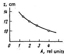
FIG. 8. Distance over which the quasistationary wave propagates without appreciable change in amplitude as a function of the initial amplitude of the low-frequency wave. The experimental conditions correspond to those in Fig. 9.
