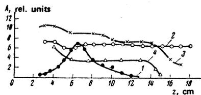
FIG. 3. Wave amplitude  $A$  as a function of distance from the point of injection of the beam for small (curve 1) and deep (curves 2, 3, 4) beam current-density modulation. For curves 1, 2, 3— $I_{b0} = 10$  mA,  $U_0 = 340$  eV; 4— $I_{b0} = 5$  mA,  $U_0 = 300$  eV;  $f = 420$  MHz, 1— $I_b/I_{b0} = 6 \times 10^{-3}$ ; 2, 3, 4— $I_b/I_{b0} \sim 1$ ; the situations corresponding to curves 2 and 3 differ by bunch parameters.
