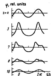
FIG. 4. Spatial evolution of the wave excited by a beam with small density modulation. The parameters of the beam-plasma system correspond to Fig. 2a and  $z$  is in centimeters.
