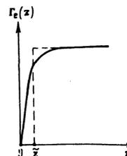
FIG. 1. The dependence  $\Gamma_e(z)$  when a new cavity appears in the Fermi surface;  $z = \tilde{m}s^2(ql)^2 \ll \tilde{m}s^2$ ;  $\Gamma_e$  is given by formula (8).
