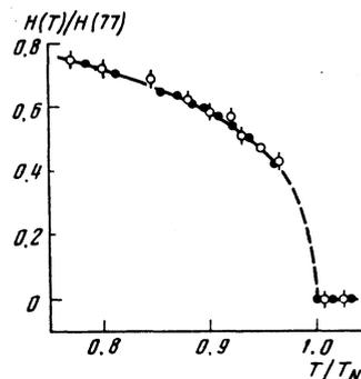
FIG. 2. Temperature dependences of the hyperfine magnetic fields at the  $^{57}\text{Fe}$  nuclei (dark circles) and  $^{119}\text{Sn}$  (light circles) in relative coordinates.
