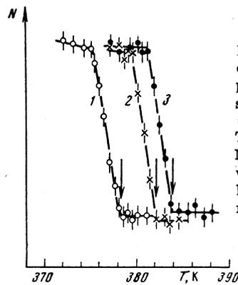
FIG. 4. Plots of the pulse counting rates against temperature at different pressures: 1— $p = 1$  atm, 2— $p = 2$  kbar, 3— $p = 3.2$  kbar. The arrows indicate the Neel temperatures. The velocity of the source relative to the absorber corresponds to resonance.
