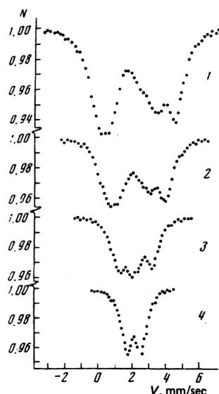
FIG. 1. Mössbauer spectra for the nuclei  $^{119}\text{Sn}$  in  $\text{FeSn}_2$ : 1-77 K, 2-291.2 K, 3-365.1 K, 4-396.8 K. The statistical errors do not exceed the dimensions of the points
