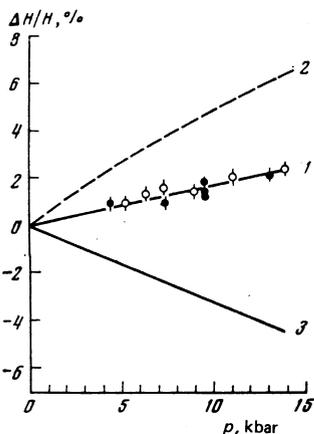
FIG. 3. Plots of the relative changes of the hyperfine magnetic fields at the nuclei  $^{57}\text{Fe}$  and  $^{119}\text{Sn}$  in  $\text{FeSn}_2$  on the pressure at room temperature: 1—experiment (dark circles— $^{57}\text{Fe}$ , light circles— $^{119}\text{Sn}$ ), 2—calculation with only the influence of  $T_N(p)$  taken into account, 3—result of subtracting the ordinates of lines 1 and 2.
