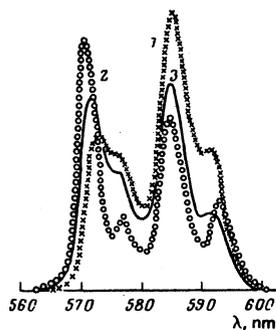
FIG. 6. Luminescence excitation spectrum for  $\text{Nd}^{3+}$  in LGS-28-0.3 glass at different delay times  $t_d$  (curve 1,  $t_d = 10 \text{ sec}$ ; curve 2,  $t_d = 3 \text{ msec}$ ) and the absorption spectrum at the  ${}^4I_{9/2} - ({}^4G_{5/2}, {}^2G_{7/2})$  transition (curve 3) at  $77^\circ\text{K}$ .
