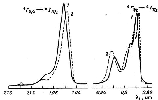
FIG. 3. Luminescence spectra of type LGS-28 silicate glass under selective laser excitation ( $T = 77$ °K); curve 1 (the full curve) is for  $\lambda_e = 575$  nm, and curve 2 (the dashed curve), for  $\lambda_e = 568$  nm.
