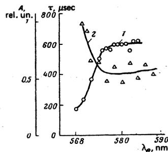
FIG. 7. Average delay time  $\tau_{\text{av}}$  for the luminescence from the  ${}^4F_{3/2}$  level of  $\text{Nd}^{3+}$  (curve 2) and the radiative transition probability  $A({}^4F_{3/2} - {}^4I_{9/2})$  (curve 1) vs exciting-light wavelength  $\lambda_e$ .
