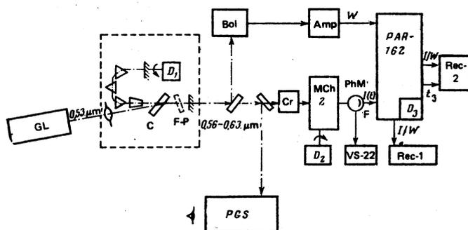
FIG. 2. Diagram of the apparatus: GL—type LTIPCh-7 garnet laser with neodymium, Bol—bolometer, Amp—amplifier, PGS—spectrograph, Cr—cryostat, MCh—type MDR-2 monochromator, PhM—type FEU-83 photomultiplier, PAR-162—boxcar integrator, Rec-1—type EPP-09 plotter, Rec-2—type PDS-021 recorder.
