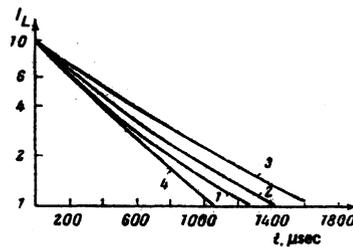
FIG. 5. Decay curves for the luminescence from the  ${}^4F_{3/2}$  level of  $\text{Nb}^{3+}$  in LGS-28-0.3 glass under selective laser excitation ( $T=4.2^\circ\text{K}$ ); curves 2-4 are for  $\lambda_e=466, 567, 568,$  and  $573$  nm, respectively.
