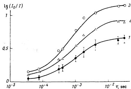
FIG. 2. Depth of valley in the dye-laser generation spectrum as a function of generation time for three different water-vapor lines with different equivalent widths<sup>[24]</sup> for the solar spectrum: 1— $\lambda=5906$ , 30 Å,  $\Delta\lambda=2\times 10^{-3}$  Å; 2— $\lambda=5907.48$  Å,  $\Delta\lambda=3.0\times 10^{-3}$  Å; 3— $\lambda=5908.21$  Å,  $\Delta\lambda=9.5\times 10^{-3}$  Å.
