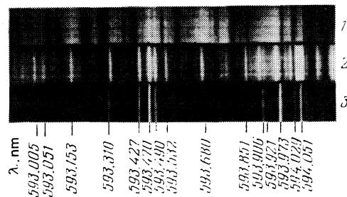
FIG. 3. Spectrum of NO<sub>2</sub> obtained with a continuously-operating dye laser for different NO<sub>2</sub> concentrations in the atmosphere: 1— $10^{-8}$  atm; 2— $2\times 10^{-7}$  atm; 3— $10^{-5}$  atm.
