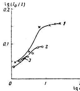
FIG. 5. Depth of valley on the  $\text{CO}_2$  lines in the generation spectrum of the  $\text{Nd}^{3+}$  glass laser for different generation times and different  $\text{CO}_2$  partial pressures: 1—0.05 atm, 2—0.016 atm, 3—0.006 atm. Measurements were performed for the  $j=14$  line associated with the  $(04^03 - 00^00)$  vibrational transition in the *R* band of  $\text{CO}_2$ .
