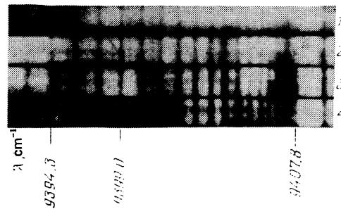
FIG. 4. Absorption spectrum of  $\text{CO}_2$  in the atmosphere, obtained with the aid of an  $\text{Nd}^{3+}$  glass laser with different generation times: 1— $5 \times 10^{-4}$  sec; 2— $1.3 \times 10^{-3}$  sec; 3— $5 \times 10^{-3}$  sec; 4— $10^{-2}$  sec. Partial pressure of  $\text{CO}_2$  is 0.05 atm for all the spectra.
