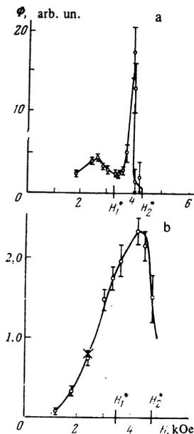
FIG. 4. Probability of interaction of two magnons of different frequencies as a function of magnetic field ( $\nu_m = 35.73$  GHz): a,  $\nu_p = 26.30$  GHz,  $H_1^* = 3.25$  kOe,  $H_2^* = 4.27$  kOe; b,  $\nu_p = 29.83$  GHz,  $H_1^* = 3.50$  kOe,  $H_2^* = 4.88$  kOe;  $T = 1.6$  K (the cross shows a value at  $T = 2.1$  K).
