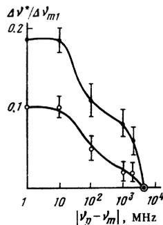
FIG. 5. Variation of the turned off part of the relaxation,  $\Delta\nu^*$ , with the difference of pumping frequencies:  $\nu_m = 35.73$  GHz,  $h_p/h_{p2} = 1.05$  to 1.25;  $\circ$ ,  $H = 2.4$  kOe;  $\bullet$ ,  $H = 1.2$  kOe.
