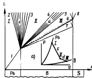
FIG. 2.  $x-t$  and  $P-U$  diagrams (a) of release wave with evaporation taken into account. Constant flow regions: I—initial state, II—phase boundary, III—final state;  $c$ ,  $d$ —centered release waves. 1— $D_{Pb}$ , 2— $U_I - C_{II}^L$ , 3— $U_{II} - C_{II}^L$ , 4— $U_{II} - C_{II}^{L+G}$ , 5— $U_{III} - C_{III}^{L+G}$ , 6— $U_{III}$ , 7— $D_A$ , 8— $D_S$ ;  $D$  and  $U$  are the wave and mass velocities,  $C$  is the speed of sound, A—air, S—screen.
