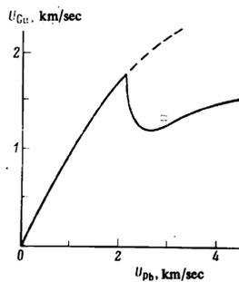
FIG. 4. Mass velocity in copper screen when lead is stopped. Solid line—calculation with allowance for evaporation, dashed—stopping of metastable liquid, □—our experiment.
