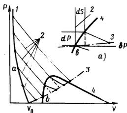
FIG. 1.  $P-V$  diagram of the experiment: 1—shock adiabat, 2—release isentropes (the metastable isentropes are shown dashed), 3—final-state curve in the case of release in air, 4—boundary of liquid-vapor two-phase region.
