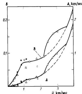
FIG. 3. Deviation from the doubling law in isentropic expansion of lead in air. Equilibrium and metastable (dashed) expansion at  $P_{in,air} = 1$  bar ( $\Delta = W - 2U$ ,  $\delta = \Delta/2U$ );  $\circ$ —our results,  $\bullet$ —<sup>[18]</sup>,  $\Delta$ —<sup>[19]</sup>.
