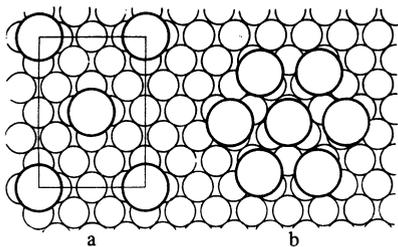
FIG. 1. Models of commensurate (a) and incommensurate (b) structures of a strontium film adsorbed on the (011) face of molybdenum: a)  $c(3 \times 3)$ ; b) hexagonal.
