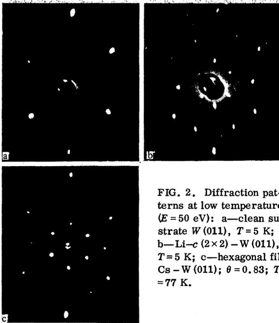
FIG. 2. Diffraction patterns at low temperatures ( $E = 50$  eV): a—clean substrate  $W(011)$ ,  $T = 5$  K; b— $Li-c(2 \times 2)-W(011)$ ,  $T = 5$  K; c—hexagonal film  $Cs-W(011)$ ;  $\theta = 0.83$ ;  $T = 77$  K.
