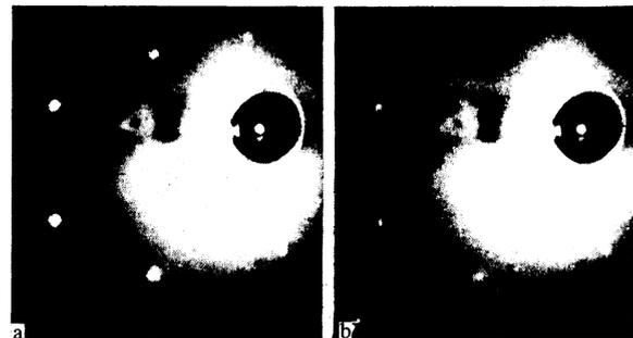
FIG. 4. Diffraction patterns of hexagonal  $La$  film adsorbed on the face  $(011)W$  ( $\theta = 0.75$ ;  $E = 33$  eV) at different temperatures: a— $T = 300$  K; b— $T = 940$  K.
