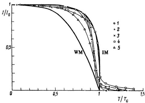
FIG. 5. Temperature dependences of the intensities of superstructure reflections of commensurate films: 1–5—for the same systems as 1–5 on Fig. 3; IM and WM—calculations for the Ising and Weiss models, respectively.<sup>[25]</sup>
