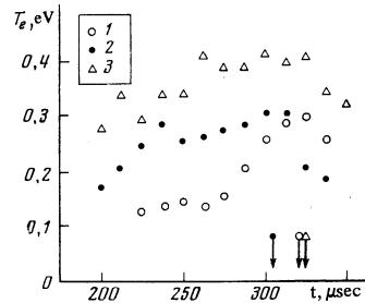
FIG. 3. Time dependence of the plasma-electron temperature at various  $H_2$  contents in the helium-hydrogen mixture (experiment).  $1—N_{H_2} = N_{He}$ ,  $2—N_{H_2} = \frac{1}{3}N_{He}$ ,  $3—N_{H_2} = \frac{1}{9}N_{He}$ .  $N_{He} = (2-4) \cdot 10^{18} \text{ cm}^{-3}$  and  $\nu_i \approx 100-200 \text{ sec}^{-1}$  everywhere. The time is reckoned from the instant when the electron beam is turned on, and the instants of the beam shutoff are marked by arrows.
