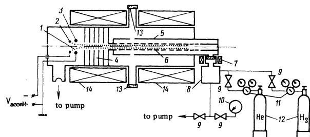
FIG. 1. Experimental setup: 1—electron beam, 2—annular cathode, 3—accelerating electrode, 4—gas delay line, 5—outer tube, 6—inner tube that limits the working volume, 7—electromagnetic valve, 8—volume ahead of valve, 9—valve, 10—manometer, 11—pressure reducer, 12—gas flasks, 13—windows for spectroscopic diagnostics, 14—magnetic-field coils.
