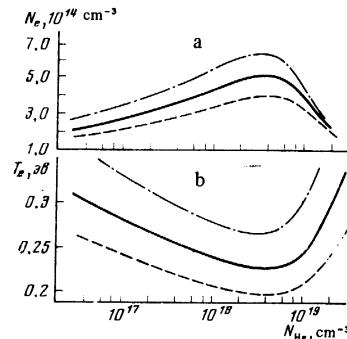
FIG. 4. Plasma density (a) and electron temperature (b) as a functions of the helium concentration at various  $H_2$  contents in the helium-hydrogen mixture (calculation). (—)  $N_{H_2} = N_{He}$ , (—·—)  $N_{H_2} = \frac{1}{2} N_{He}$ , (—·—·—)  $N_{H_2} = \frac{1}{4} N_{He}$ . We put through-out  $v_i = 200 \text{ sec}^{-1}$  and  $T = 0.1 \text{ eV}$ .
