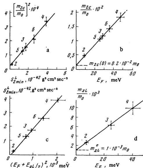
FIG. 2. The dependence (a) of the cyclotron mass  $m_{2c}$  on  $S_{2\text{min}}^L$  and (b) on  $E_F$ , (c) of  $S_{2\text{min}}^L$  on  $(E_F + E_{gL}/2)^2$ , and (d) of  $m_{xL}$  on  $E_F$  for carriers at the  $L_a$  and  $L_s$  extrema in  $\text{Bi}_{0.924}\text{Sb}_{0.076}$  at liquid-helium temperatures. The figures indicate the sample numbers.
