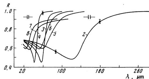
FIG. 1. Reflection spectra for doped  $\text{Bi}_{0.924}\text{Sb}_{0.076}$  at  $T = 12$  K. The figures beside the curves correspond to the numbers of the samples in the table.
