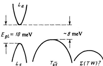
FIG. 3. Diagram of the arrangement of the main extrema in  $\text{Bi}_{0.924}\text{Sb}_{0.076}$ .
