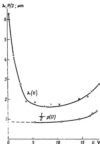
FIG. 3. Dependence of the texture periodicity  $\lambda$  and of the helix half-pitch  $P/2$  on the voltage  $U$ ;  $L = 15 \mu\text{m}$ ;  $P_0 = 1.7 \mu\text{m}$ . The total untwisting of the helix takes place at a voltage  $U_{c-N} = 25 \text{ V}$ .
