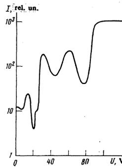
FIG. 4. Dependence of the intensity of the transmitted light  $I$  on the voltage  $U$  on the cell.  $L = 60 \mu\text{m}$ ;  $P_0 = 1.7 \mu\text{m}$ .
