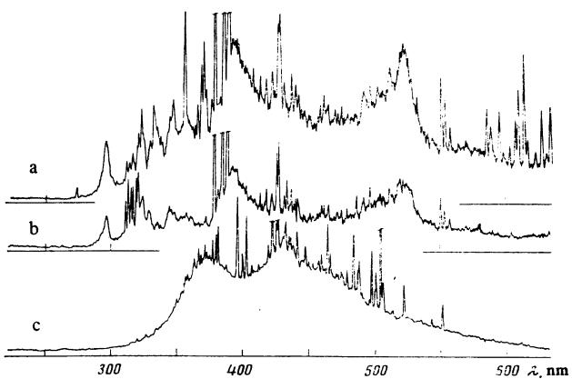
FIG. 2. Segments of the emission spectra recorded for molybdenum bombarded by neon (a) and argon (b) ions, and for tungsten bombarded by argon ions (c). Ion energy 12 keV; beam current density  $2 \times 10^{-4}$  A/cm $^2$ ; residual-gas pressure  $10^{-7}$  Torr.
