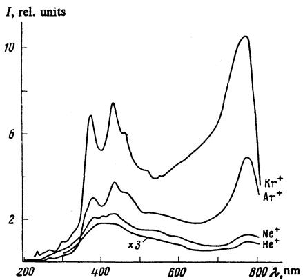
FIG. 3. Intensity distribution in the continuous spectrum recorded for tungsten bombarded by helium, neon, argon, and krypton ions (ion energy 12 keV; beam current density  $0.6 \times 10^{-4}$ – $2 \times 10^{-4}$  A/cm $^2$ ). Data corrected for the spectral sensitivity of the radiation-detecting system.
