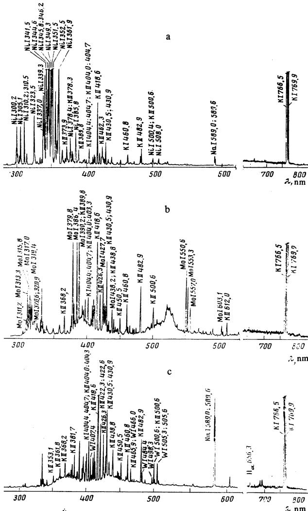
FIG. 1. Emission spectra recorded for nickel (a), molybdenum (b), and tungsten (c) bombarded by 12-keV potassium ions. Beam current  $10^{-3}$  A/cm $^2$ ; residual-gas pressure  $\sim 5 \times 10^{-8}$  Torr.
