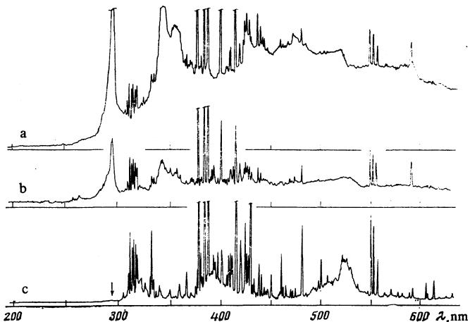
FIG. 4. Emission spectra obtained for molybdenum bombarded by potassium ions (ion energy 12 keV; beam current density  $0.2 \times 10^{-3}$  A/cm $^2$ ) at the following residual-gas pressures: a)  $\sim 2 \times 10^{-6}$  Torr; b)  $\sim 5 \times 10^{-7}$  Torr; c)  $\sim 5 \times 10^{-8}$  Torr.
