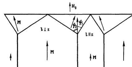
FIG. 3. Structure of the intermediate state of antiferromagnets when  $\beta \rightarrow 0$ .
