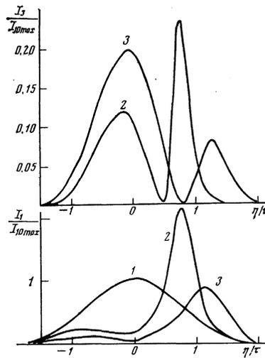
FIG. 2. Evolution of the pumping and third-harmonic pulses at  $\theta_0 = 2.2\pi$  and  $|\beta| = 0.5$ : 1—pulses at the entrance; 2, 3—pulses at  $z = l_n$  and  $z = 2l_n$ .
