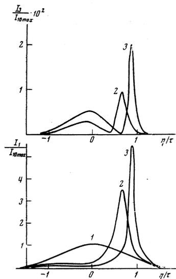
FIG. 1. Evolution of the pumping and third-harmonic pulses at  $\theta_0 = 2.2\pi$  and  $|\beta| = 0.06$ : 1—pumping pulse at the entrance; 2, 3—pulses at  $z = l_n$  and  $z = 2l_n$ .
